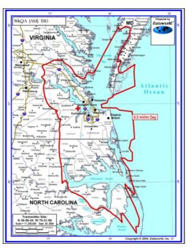
**WKQA** is a 50,000-watt clear-channel station that broadcasts from Norfolk, Va., with a listenership that extends farther than the red outline shown on the map.
